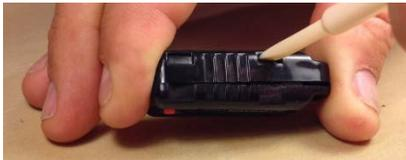
Then, on the side most convenient to you, gently push in (just a little) and down on one tab until you feel a slight gap open up in the case. Don't try to completely push the tab in! Just push it in a little to unhook it and keep the gap open with the hand that is clamping the ends. Do the same thing for the other tab on that side so that both tabs are unlatched.
