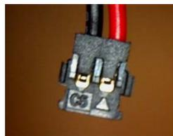
To reconnect, align the correct side of the plug to the connector on the board, and then snap it in by pressing it down into the board. When snapped in, it will be completely snapped into the connector. It should look like this when you are done:
