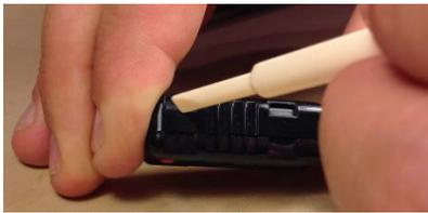
Once both tabs on one side are unlatched, you can then widen the gap and open the case.
